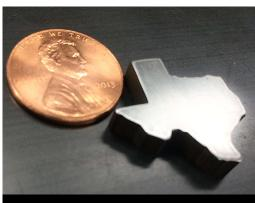
Wire EDM used to cut complex shapes with a high degree of accuracy. This process can be used with all types of metals from aluminum and brass to carbide and inconel.
